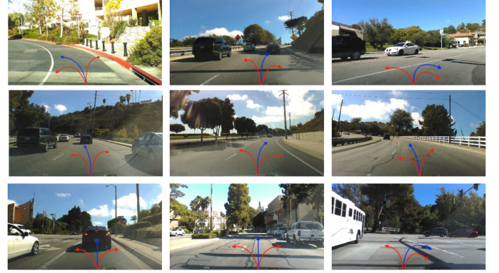
Figure 4: Single-bit flip outcome on the self-controlled steering systems. Blue arrows point to the expected steering angles and red arrows are faulty outputs by the systems.
